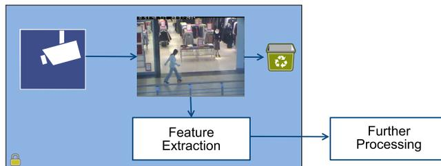
Fig. 4: A feature-camera (blue frame) captures images, computes local features and only exports the features.
