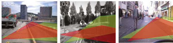
Fig. 5. Improvement of ground plane estimation performance. Particle MCMC improved qualitative accuracy of ground plane estimation, where red and green planes denote ground planes obtained by Particle MCMC and Gibbs sampling, respectively.
